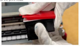
• Let's cap the printhead side with the smaller transparent caps. Push the caps until the first rib on the nozzle. Then close the lid.
