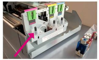
Let's cap the printhead side with the smaller orange caps. Push the caps until the first rib on the nozzle. Then close the lid.
