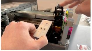
Install the red cap. Align the pins with the holes on the top of the print head.
