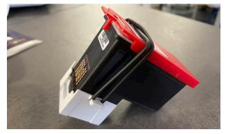
Then seal the print head by capping with a cartridge/printhead garage or put it into a properly sealed plastic box. Please do not re-tape or cover the nozzles!
