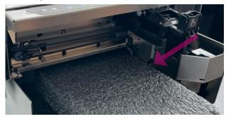
Secure the printhead with tape.
