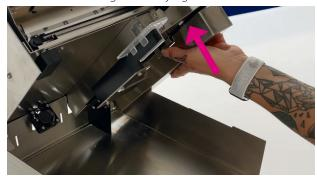
• Install the protection foam and make sure the arm fits into the cut-outs.
