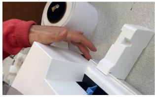
Remove the ink cartridge. Then secure the carriage with tape and insert the foam inlay.
