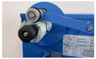
Put the slitting station in transport position.
