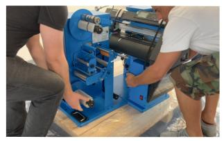
Align the fixation holes with the holes in the pallet.
