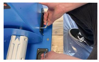
Tighten the fixation screws.
