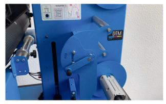
Pull down the pinch lever and secure it with tape.
