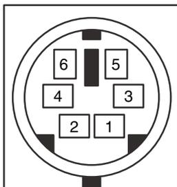
Uses 5v logic @ 5mA - All signals are active low.
