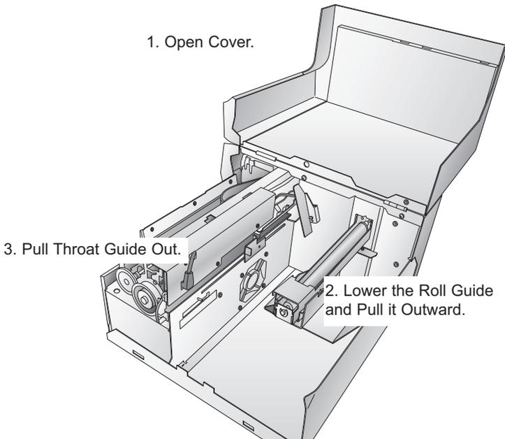
4. Remove any shipping tape from your label stock roll to ensure that it can unroll freely, making certain that no adhesive portion is exposed. It is important to note that any exposed adhesive surface can attach itself to the inner workings of the print mechanism and cause a media jam.
