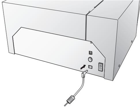
Once the power cord is connected, the printer can be switched on and off using the power switch.
