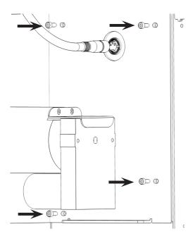
Place the liner module in correspondence to the designed holes on LF140e lateral side and secure it in place using the four allen screws. Ensure that the plug is connected properly.
