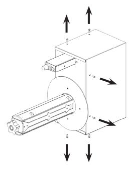
On the liner rewinder module, remove the 6 screws as shown in the picture. Than it will possible to keep out the cover.
