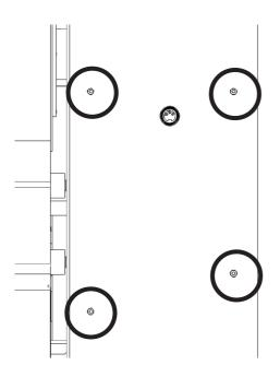
Using the supplied allen key, remove the four allen screws from LF140e lateral side
