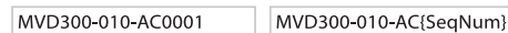
An example of a Serial Number field viewed with Field Codes off (left), and Field Codes on (right).
