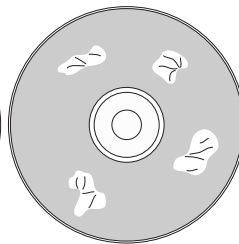
Uneven coverage due to inadequate heat
