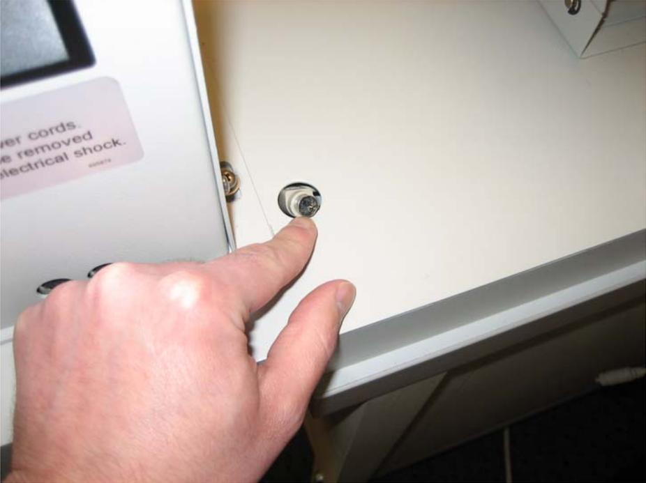
4. Disengage the feeder switch (1) and disconnect the 6-pin cable from the tension unit (2).
