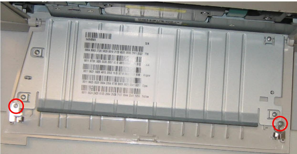
3. Be sure to remove the correct screws. The correct screws to remove are those that hold down the metal door catch. When removing the screws make sure the catches remain in the same positions. The bracket is installed over the catches.
