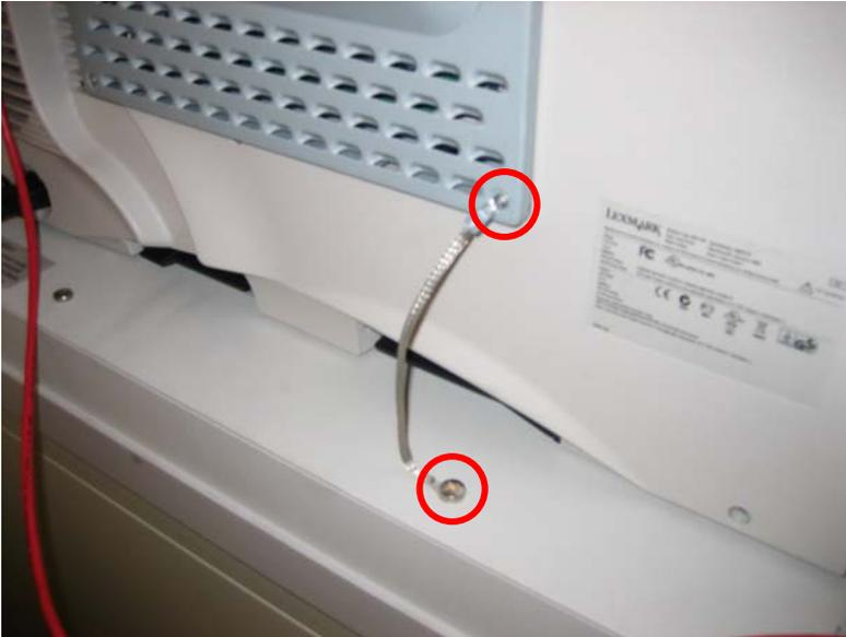
2. Install the longer grounding strap on the unwinder as shown. Remove screws on the base frame and the unwinder. Replace screws when the grounding strap is in place.
