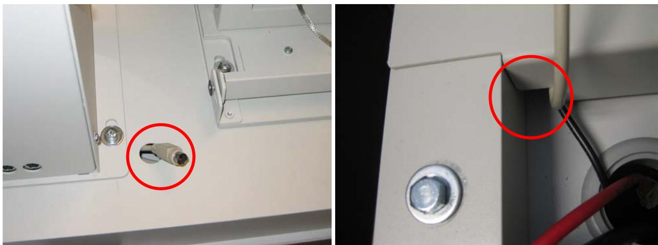
5. Reconnect the 6-pin cable to the tension unit. The flat side should be facing toward the rewinder.
