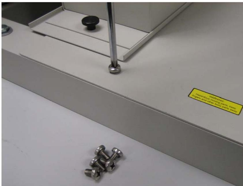
7. Pull the base plate to the side approximately 1 inch (2.5 cm) or enough so that you are able to create an overlap edge that you can grasp when lifting the plate with the rewinder and tension unit still attached.
