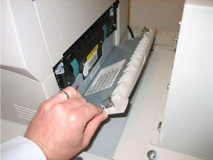
2. Remove two #2 Phillips screws as shown below.
