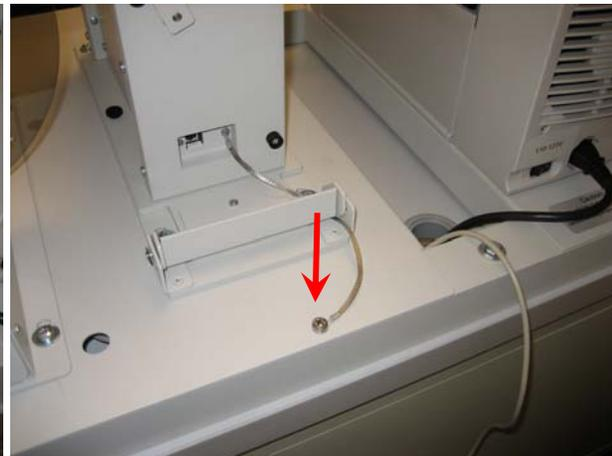
4. Feed the new 6-pin cable through the hole in the base plate and the notch on the angled portion near the printer. If you have the Primera CX1200e table you can access the notch and the hole from underneath.
